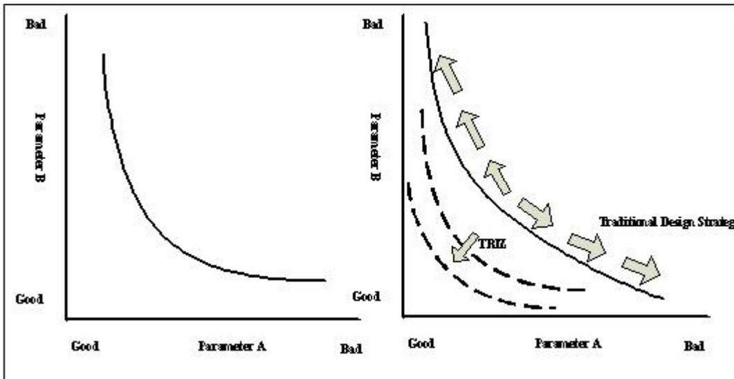
Figure 3 : How a technical contradiction happens and how TRIZ can be used to solve it (Mann, 2002)
