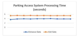
Based on the test results, the average processing time for the parking access system is  $3.88 \pm 0.07$  seconds for the entrance gate and  $5.37 \pm 0.03$  seconds for the exit gate. To check the security of the parking access system, a performance analysis is carried out based on four quadrants, as follows:
