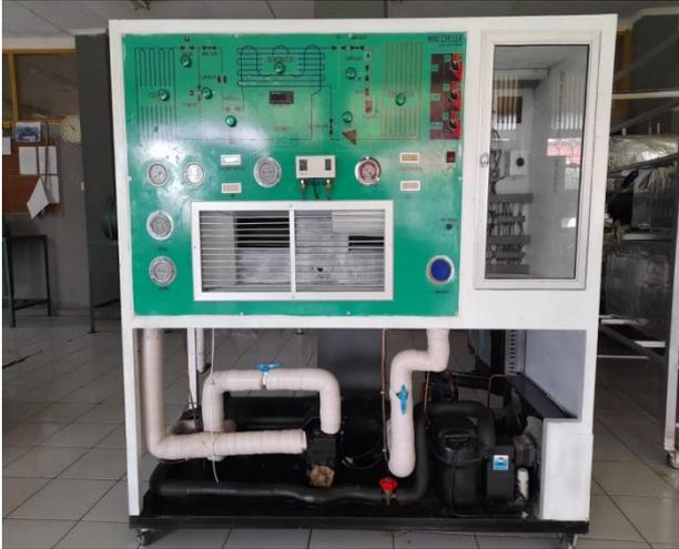
Gambar 5. Mesin Pendingin Mini Chiller
