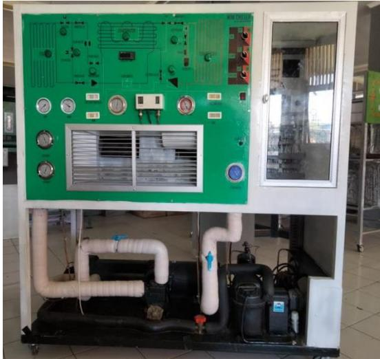
Gambar 2 Alat Uji Mini Chiller
