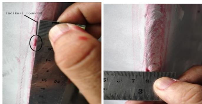
Gambar 3.3 Indikasi *Rounded* Pada *Penetrant joint* J02
