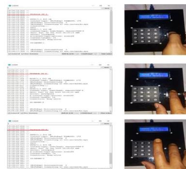
Gambar 2. Hasil Uji Arduino Mega Dengan Sensor Fingerprint Dan LCD
