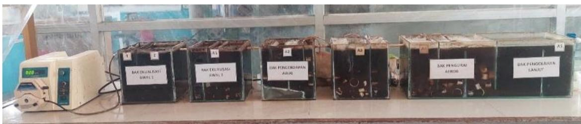
**Gambar 1** Prototype Instalasi Pengolahan Air Limbah (IPAL) Industri CPO
