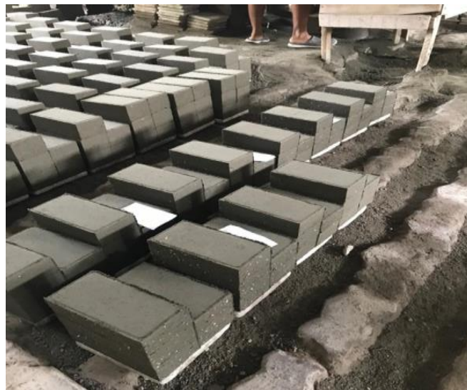
Gambar 2. Hasil paving block penambahan limbah plastik LDPE
