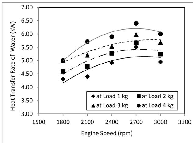
Figure 4. Heat transfer rate of water against engine speed
