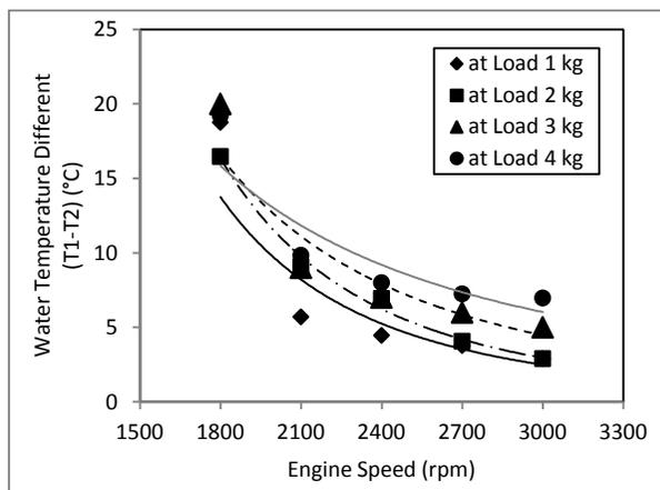
Figure 2. Water temperature different against engine speed
