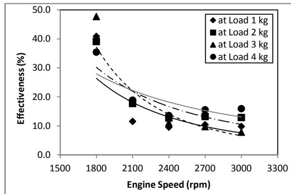
Figure 6. Heat transfer effectiveness against engine speed with loads variation
