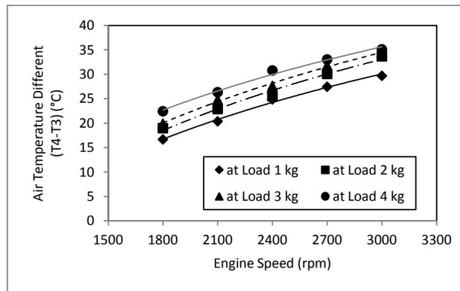
Figure 3. Air temperature different against engine speed
