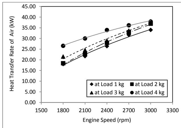
Figure 5. Heat transfer rate of air against engine speed
