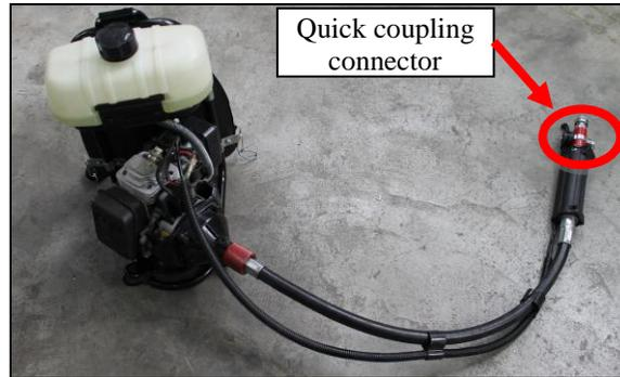
(a) The engine as the main prime mover for the tool set.
