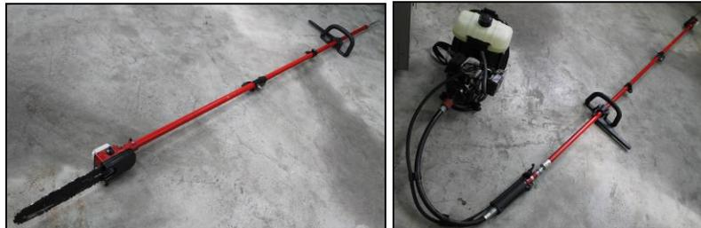
(b) The engine connected to a long pole pruner.
