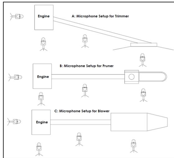
Figure 2. Microphone positions for sound pressure level measurement for each of the garden tool configuration.
