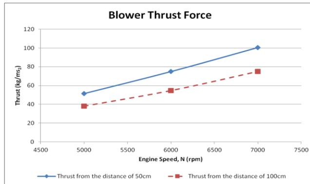
Figure 4. Blower thrust versus engine speed in two different distances.
