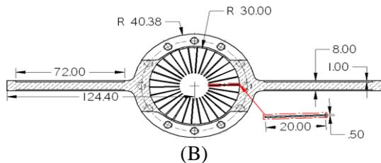
Figure 3: (A) 3D model of the heat exchanger showing the internal fins and the two extended surfaces with the machined slots for thermoelectric modules (B) A sectional side view showing the basic dimensions (in mm) of the heat exchanger.
