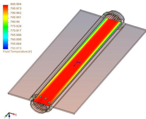
Figure 5. A cut plot showing air temperature distribution at air flowrate of 0.058 Kg/s and inlet temperature of 800 K (Scale is enlarged to show the distribution pattern)
