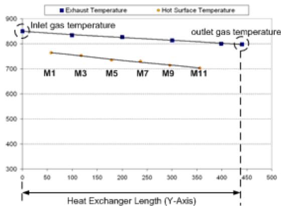
Figure 8. Exhaust gas and heat exchanger surface temperature distribution for the Nissan ETEG derived from experimental testing
