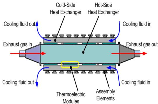
Figure 1: Schematic drawing of a typical ETEG
