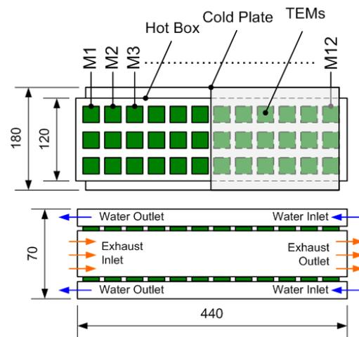
Figure 6: Schematic of Nissan ETEG showing the basic dimensions in mm
