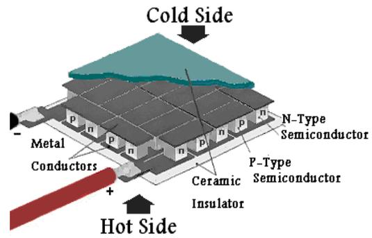
Figure 2. A cutaway drawing of a thermoelectric module showing the (P) and (N) elements
