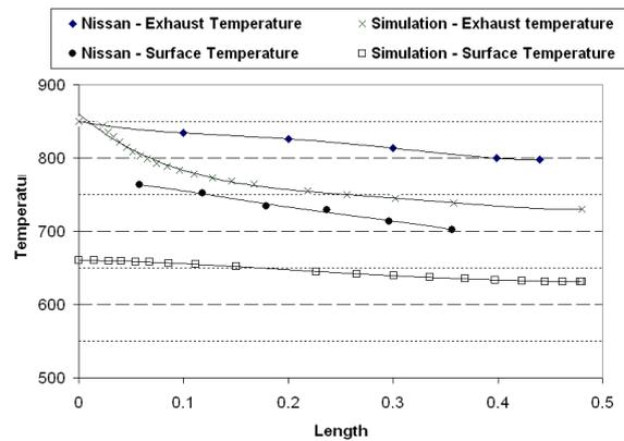
Figure 9. Comparison between the thermal performance of the simulated heat exchanger and the experimental results of Nissan ETEG.
