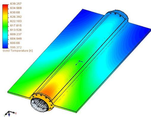
Figure 4. Solid temperature distribution at air flowrate of 0.058 Kg/s and inlet temperature of 800 K
