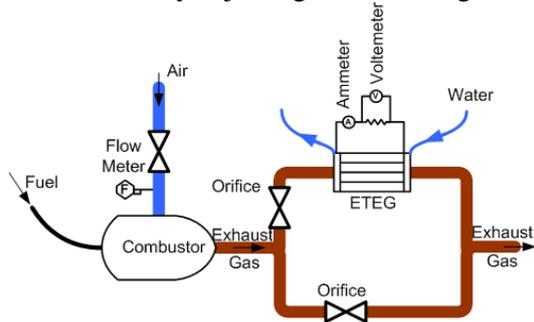
Figure 7: Schematic shows the combustor test bench used to simulate the engine exhaust for the Nissan ETEG testing
