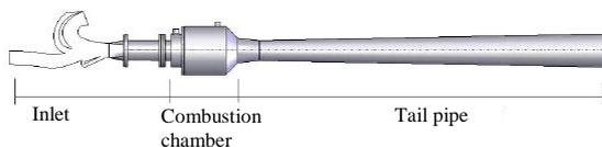
Figure 1: Pulse combustor
