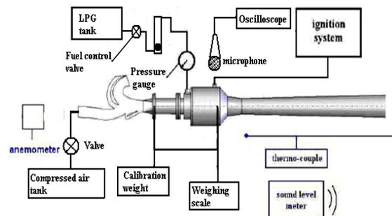
Figure 8: Experimental diagram
