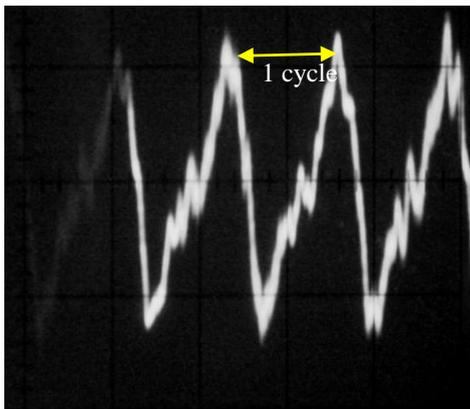
**Figure 11:** Without J-shape operating frequency, Fuel flowrate ; 50 L/m, 5ms/div
