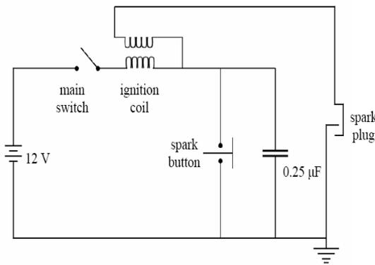
Figure 9: Ignition circuit
