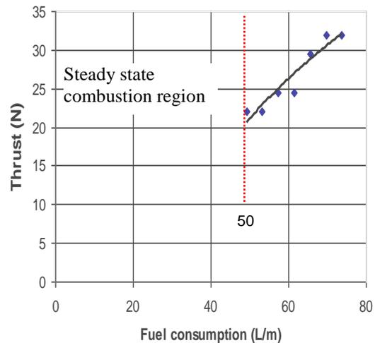
**Figure 12:** Thrust versus fuel consumption (J-shape attached)
