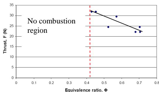
Figure 14: Thrust versus equivalence ratio
