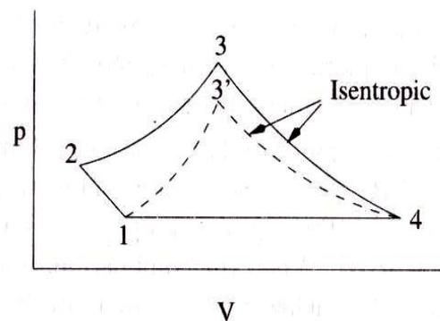
Figure 4: Pulsejet cycle on p-V diagram [Ganesan, 2005]
