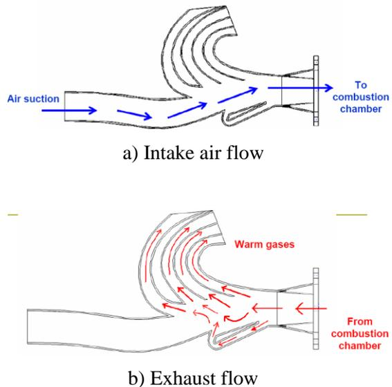
Figure 7: Flow of exhaust gas in the J-shape inlet
