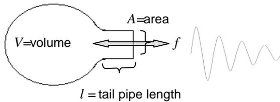
Figure 3: Helmholtz resonator
