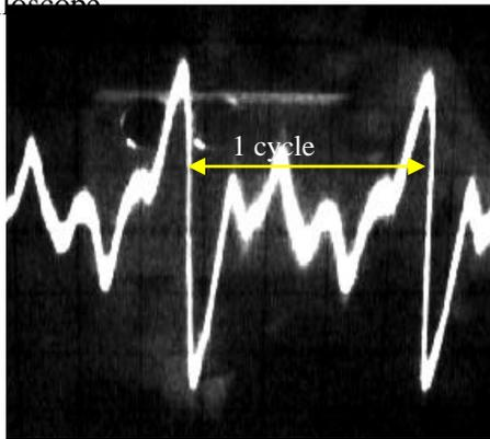
**Figure 10:** J-shape operating frequency, Fuel flowrate; 50 L/m, 3ms/div.
