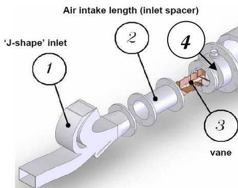
Figure 6: Inlet section
