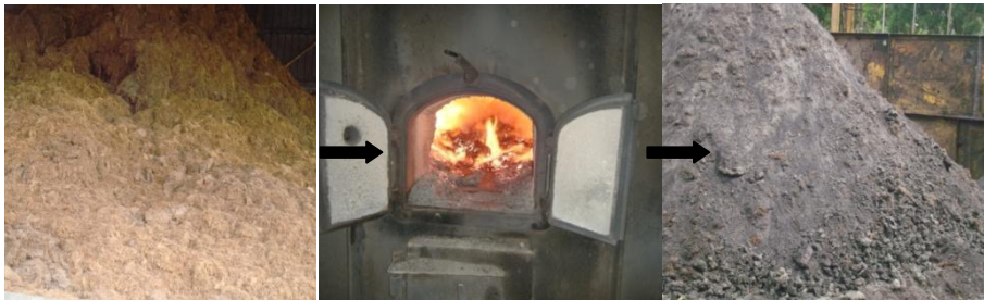
Plate 1 Heap of processed PMF Plate 2 Firing PMF and PKS Plate 3 Heap of raw POFA
