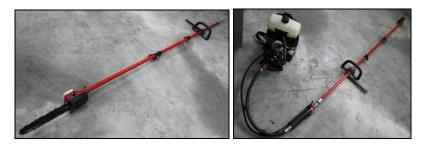
(b) The engine connected to a long pole pruner.
