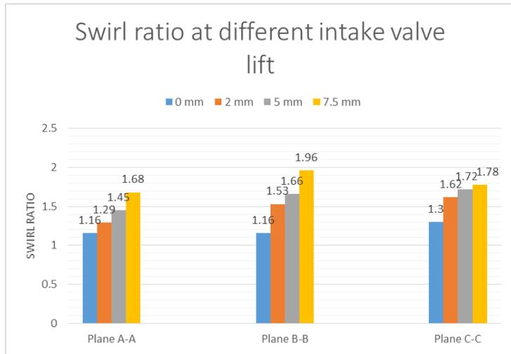
Figure 12: Swirl ratio for variation of intake valve lift at plane A-A, B-B and C-C
