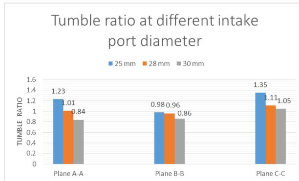
Figure 11: Tumble ratio for variation of intake port diameter at plane A-A, B-B and C-C
