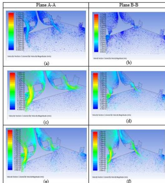
Figure 9. Velocity vectors on cut section A-A and B-B at (a) (c) (e) 7.5 mm valve lift (b) 0 mm valve lift (d) 2 mm valve lift & (f) 5mm valve lift
