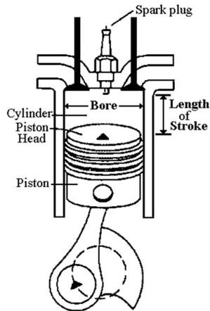
Figure 2. Bore vs length of stroke position
