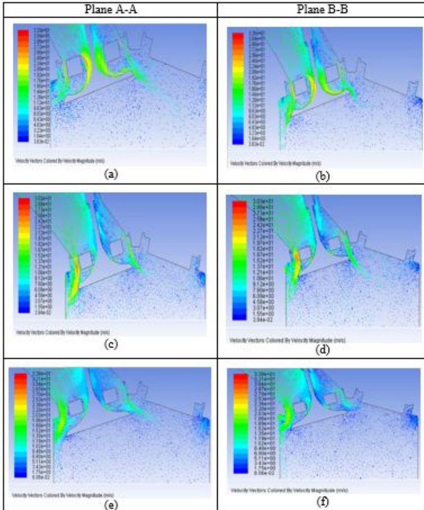
Figure 7. Velocity vector on cut section A-A and B-B at (a) (b) 25 mm intake duct, (c) (d) 28 mm intake duct & (e) (f) 30 mm intake duct
