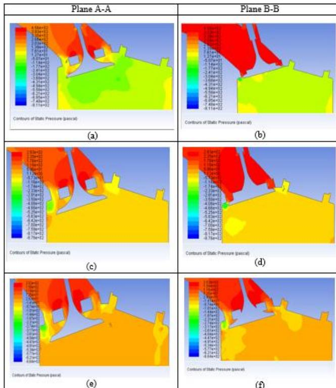
Figure 8. Pressure contours on cut section A-A and B-B at (a) (c) (e) 7.5 mm valve lift (b) 0 mm valve lift (d) 2 mm valve lift & (f) 5mm valve lift
