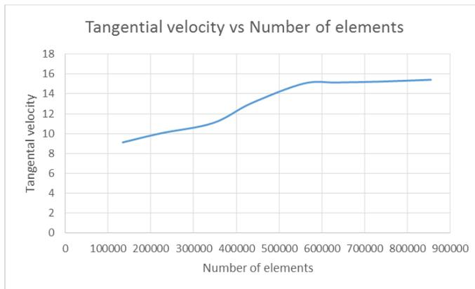
Figure 5. Graph of tangential velocity vs. number of elements
