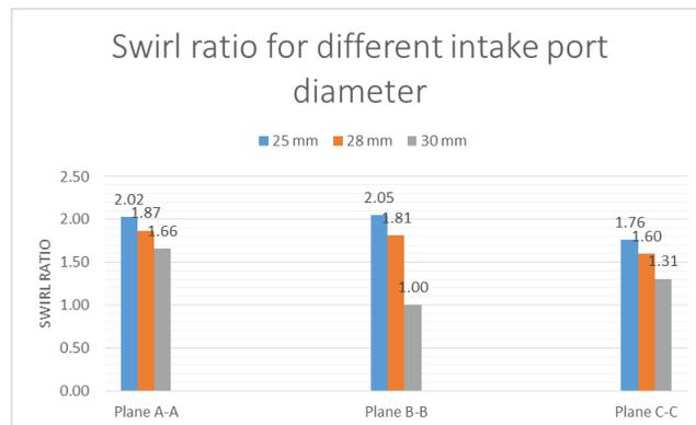
Figure 10. Swirl ratio for variation of intake port diameter at plane A-A, B-B and C-C
