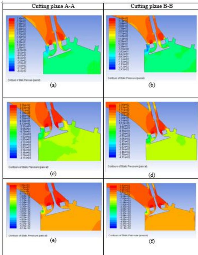
Figure 6. Pressure contours on cut section A-A and B-B at (a) (b) 25 mm intake duct, (c) (d) 28 mm intake duct, & (e) (f) 30 mm intake duct
