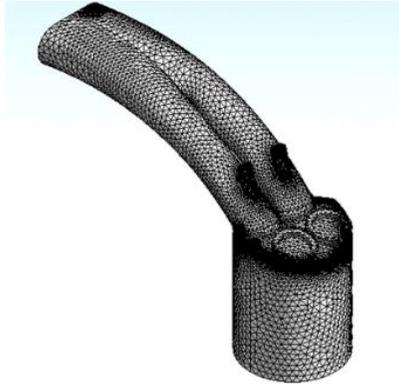
Figure 3: Mesh of 30 mm intake port diameter model
