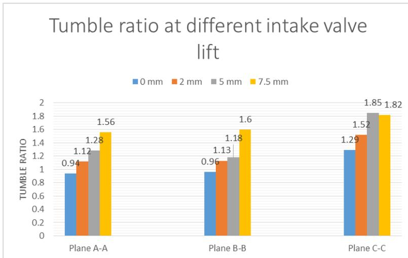
Figure 13: Tumble ratio for variation of intake valve lift at plane A-A, B-B and C-C
